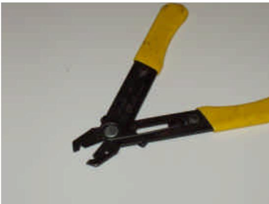
This is a less expensive wire cutter/stripper and works very well for cutting carbon fiber rods also. To make work for cutting carbon I removed the 'stop' so the 'V' cutting blade would cut small diameter rods.
