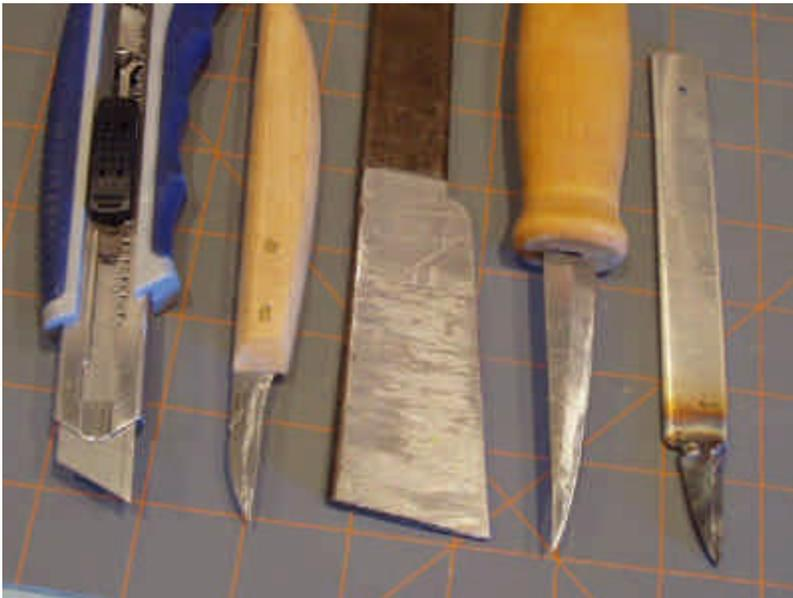
The most important aspect of working with bamboo is that the knife or tool you use, whatever type it is, is extremely sharp! Dull tools make working with bamboo very difficult to impossible.
