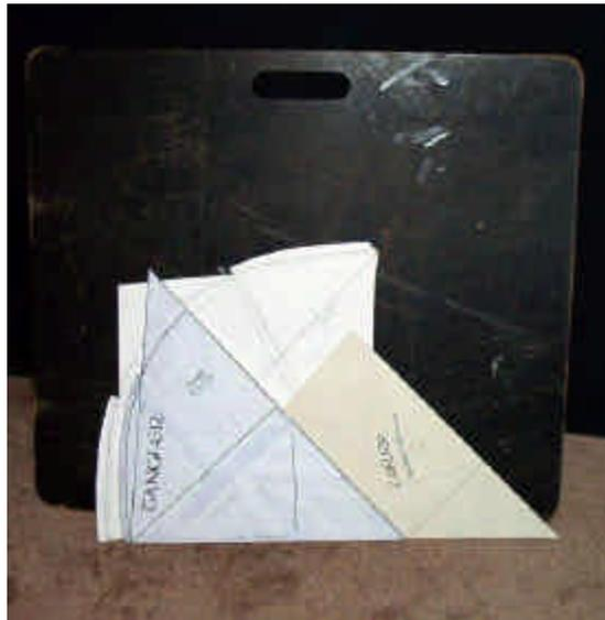
Last, I have a portable or lap board that I use for a cutting table for sails. It is made of Masonite. It has a handle for carrying, and two clips that can hold patterns when the board is not in use. When it gets a little rough, I sand the surface slightly to restore its smooth surface.
