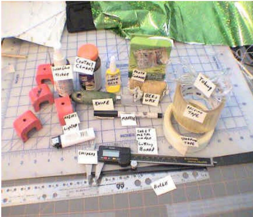
The magnets are used to hold the pattern down while cutting the sail and holding the sail while putting on the spine.
