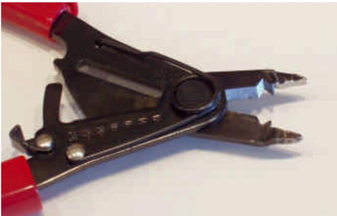
This is a wire cutter/stripper I bought for about \$9 at Home Depot. I removed the stop and filed off the teeth on the ends of the pliers so it would cut a 0.02" diameter rod in the 'V' cutter portion.
