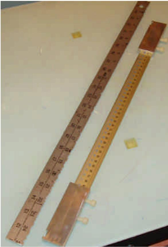
These are two different styles of bow setters I use. The one on the right is one that Manny Alves developed and made; it's adjustable. The other is an aluminum yardstick with notches filed along one edge that correspond to the wingtip locations of various kite plans I make.
